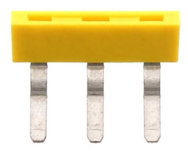
External insulated cross-connector, No. of poles: 3, Mounting type: Plug in, Width: 24.2 mm, Rated current: 27 A; Colour: Yellow
