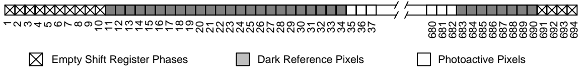
Figure 13. Line Timing Diagram – Single Register Output
