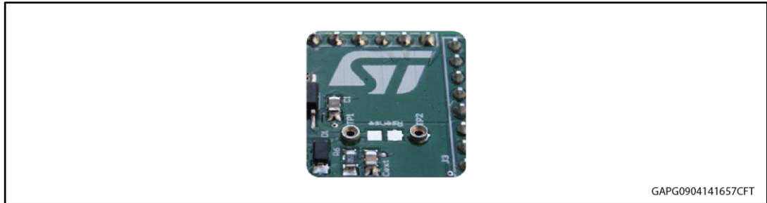
Figure 4: Mounting through-hole sense resistor
