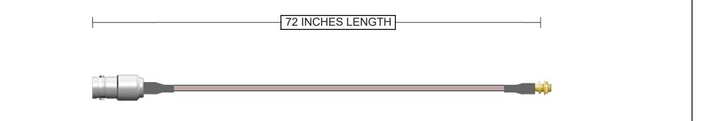
Connector A 112631 BNC Jack Straight Brass Nickel + Heatshrink 50 Ohm RG-178 Continuity/Hi-Pot Connector B 262120 MMCX Jack Straight Bulkhead - Rear Mount Brass Gold + Heatshrink
