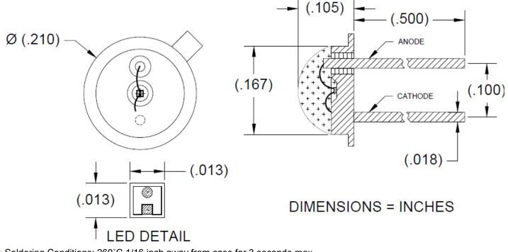
>Soldering Conditions: 260°C 1/16 inch away from case for 3 seconds max.
