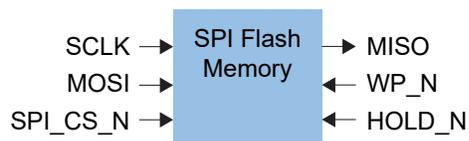
*Table 64: SPI Flash Memory Signals (Interface to FPGA Fabric)*
