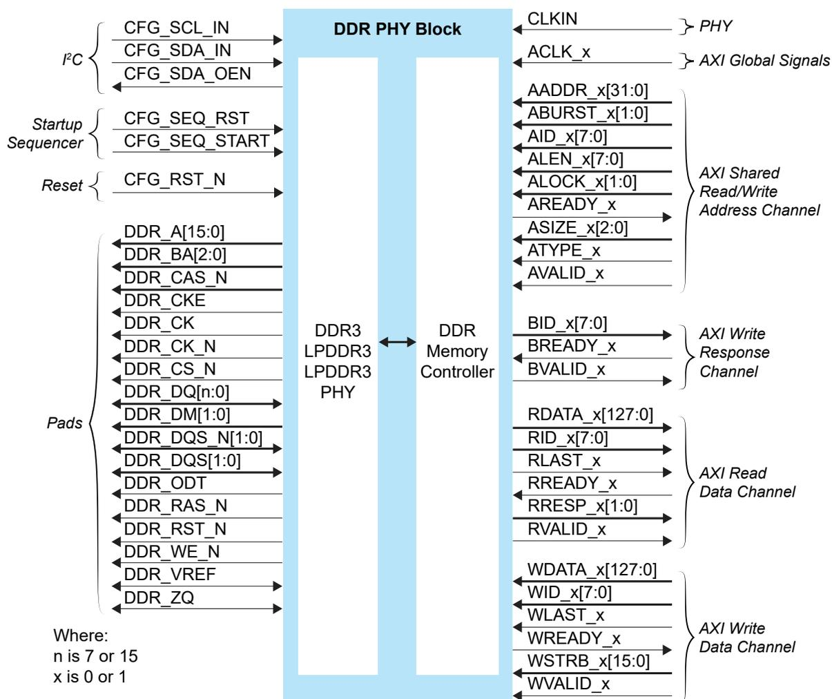
The DDR DRAM block supports an I<sup>2</sup>C calibration bus that can read/write the DDR configuration registers. You can use this bus to fine tune the DDR PHY for high performance.
