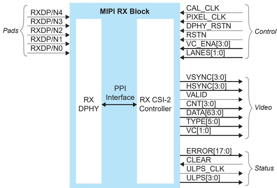
The control signals determine the clocking, how many transceiver lanes are used, and how many virtual channels are enabled. All control signals are required except the two reset signals. The reset signals are optional, however, you must use both signals or neither.
