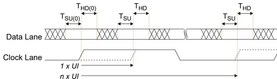
Figure 32: LVDS RX Timing (Edge-Aligned)
