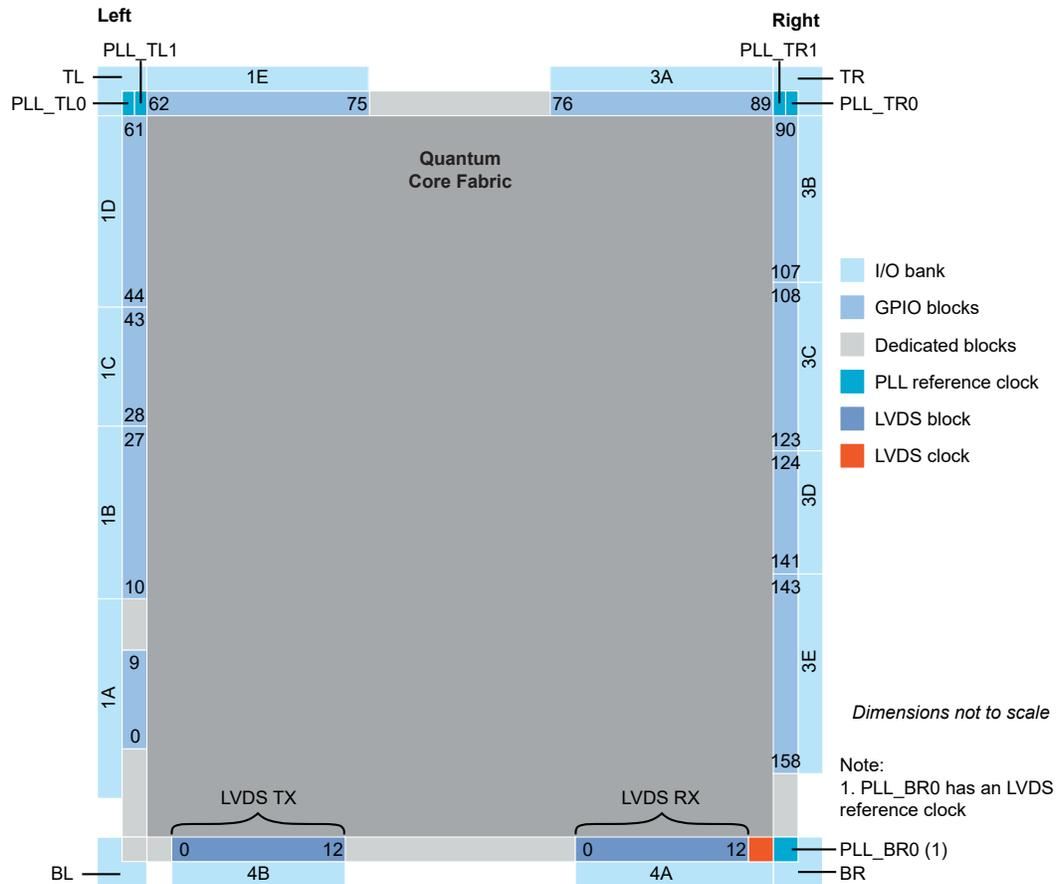
Figure 41: Floorplan Diagram for FPGAs in BGA324 Packages (with DDR and MIPI)
