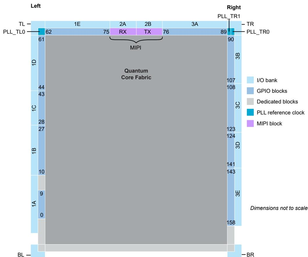
Figure 38: Floorplan Diagram for QFP100F3 and QFP144 Packages
