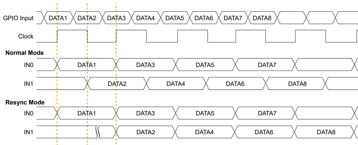
In resync mode, the IN1 data captured on the falling clock edge is delayed one half clock cycle.
