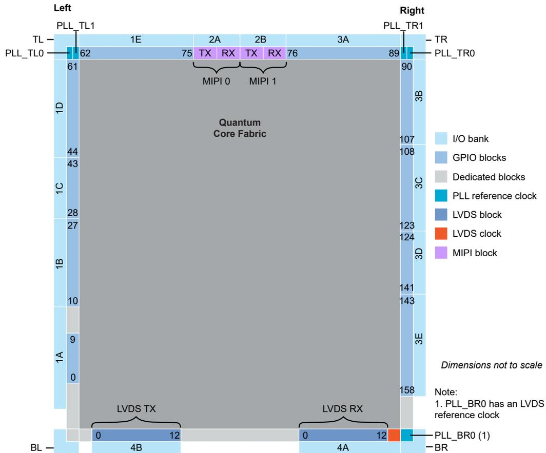
Figure 40: Floorplan Diagram for FPGAs in BGA256 Packages
