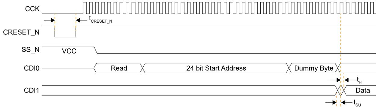
Figure 35: SPI Passive Mode (x1) Timing Sequence
