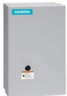
Non-reversing NEMA contactor, Size 0, Three phase full voltage, Contactor amp rating 18A, 3 wire (NO aux included), 110V 50Hz / 120V 60Hz coil, Noncombination type, Enclosure NEMA type 1, Indoor general purpose use, Extra-wide enclosure
