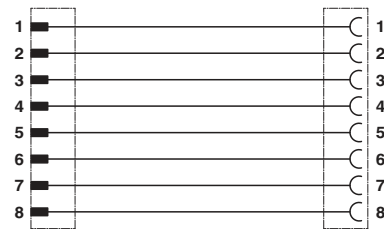
Contact assignment of M12 connector/socket
