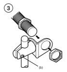
Fasten the two parts of the mounting clamp (a) loosely by means of the screw (b) and the nut (c) supplied.
