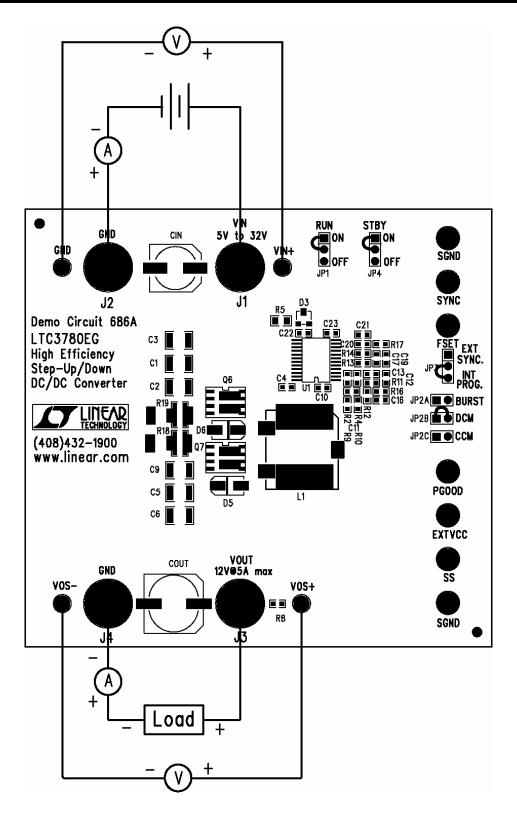
Figure 1. DC686 Test and Measurement Setup Diagram
