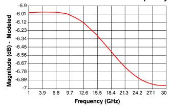
Modeled with HFSS using Rogers 3003 substrate, with a thickness of 10 mils and a line width of 24 mils, representing data for 100 Ohms.
