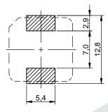
no sensitive traces underneath the component
