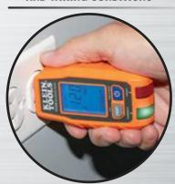
**Power button**; tester auto-powers off after 3 minutes of inactivity to conserve battery life.
