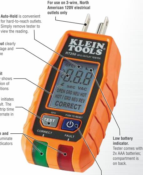
CLEAR INDICATION OF VOLTAGE AND WIRING CONDITIONS
