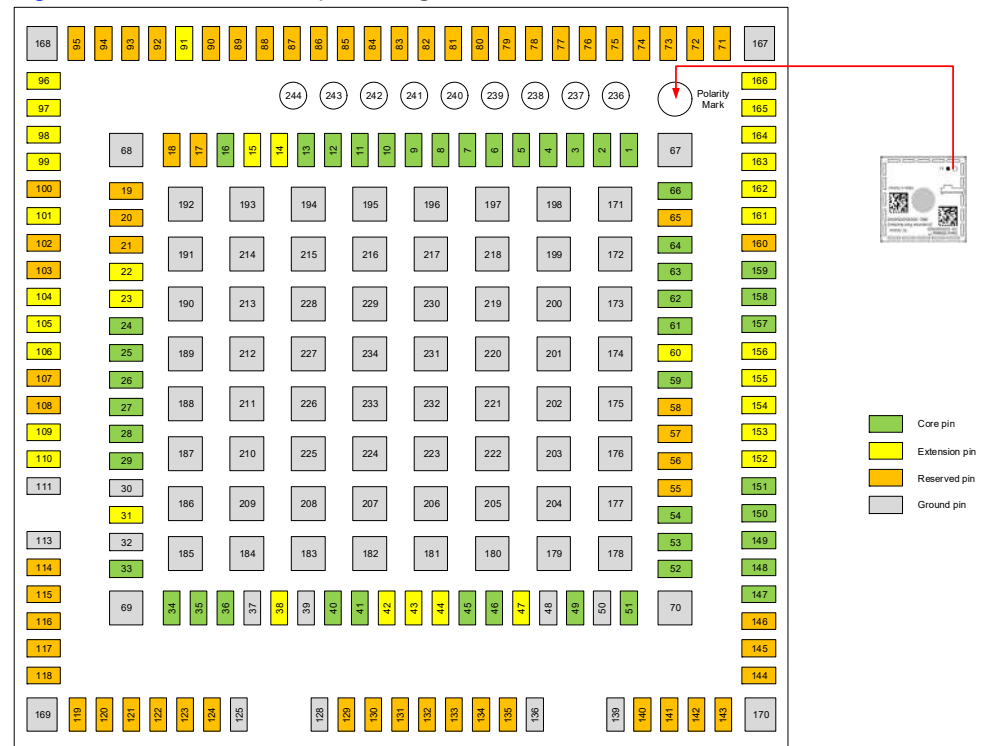
Figure 10-1: Pin Configuration (Top View, Through Module)
