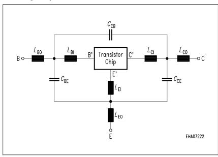
The TSFP-4 package has two emitter leads. To avoid high complexity fo the package equivalent circuit, both leads are combined in one electrical connection.
