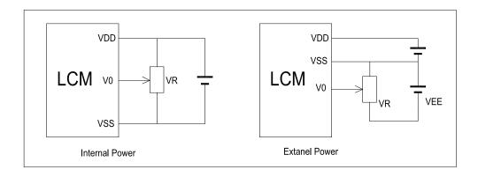
$V_{DD^{\sim}}V_0$ : LCD Driving voltage VR:  $10k^{\sim}20k$
