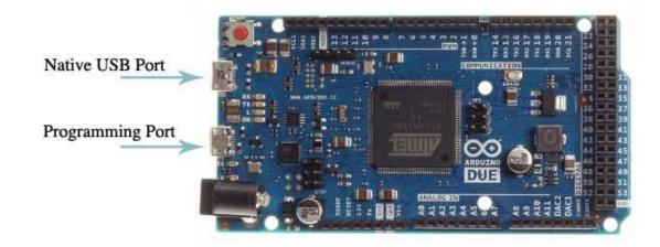
Either of the USB ports can be used for programming the board, though it is recommended to use the Programming port due to the way the erasing of the chip is handled :
