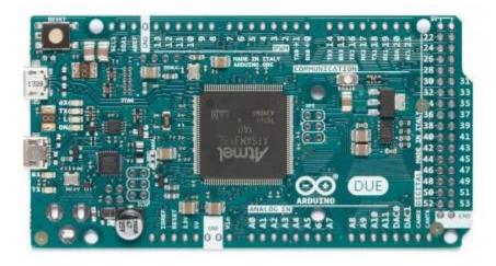
The Arduino Due is a microcontroller board based on the Atmel SAM3X8E ARM Cortex-M3 CPU. It is the first Arduino board based on a 32-bit ARM core microcontroller. It has 54 digital input/output pins (of which 12 can be used as PWM outputs), 12 analog inputs, 4 UARTs (hardware serial ports), a 84 MHz clock, an USB OTG capable connection, 2 DAC (digital to analog), 2 TWI, a power jack, an SPI header, a JTAG header, a reset button and an erase button.
