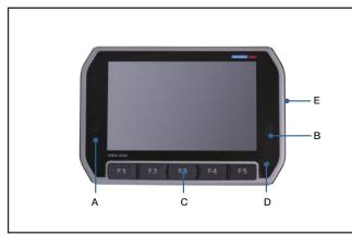
A. B. Speaker C. User-defined hotkeys D. Light sensor E. Reset, power, USB host (side)
