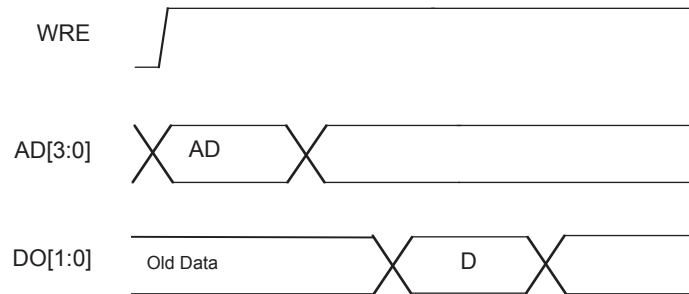
Figure 3-7. Slice Single /Dual Port Read Cycle Timing
