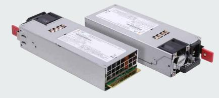
Advanced Energy's Artesyn CSU550AP power supply is housed in a 1U high rack-mount enclosure measuring just 2.89 x 7.28 inches (73.5 x 185.0 mm). This form factor is significantly narrower and shorter than that of similarly rated earlier generation power supplies — freeing up valuable system space — and is achieved by use of the latest power switching technology and high density component packaging techniques. This form factor conforms to the standard market's Common Redundant Power Supplies.
