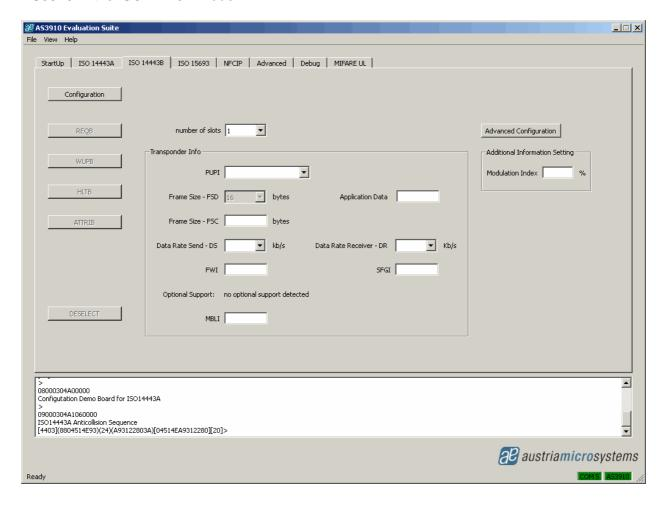
After clicking the button *Configuration*, an ISO14443B tag can be placed close to Demo board antenna. Clicking button *REQB* starts the request procedure. When REQB is terminated the PUPI number of the founded tags is displayed.
