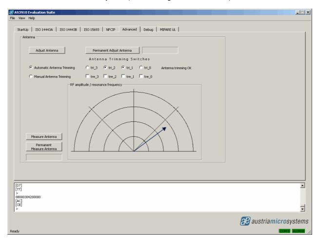
The antenna can be tuned by the button *Adjust Antenna* while *Automatic Antenna Tuning* is selected. Figure below depicts the result after clicking this button (metal was kept close to antenna). Note that position of trimming switches changed.
