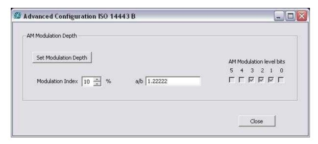
Advanced Configuration button is used to change the modulation depth. Once it is selected, an Advanced Configuration ISO14443B window pops up. After selecting the wanted modulation depth, it is set by the Set Modulation Depth button.
