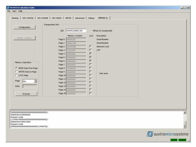
To write data, radio button "WRITE Data to Page" and the wanted Page have to be selected and the data placed in the Data field (4 bytes).
