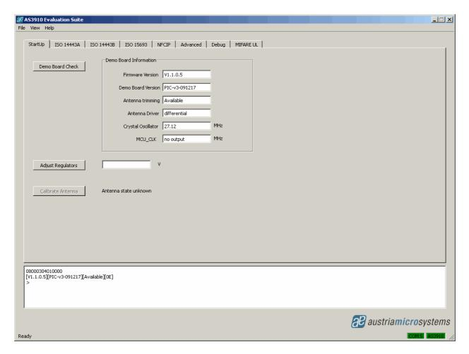
Figure above depicts the GUI window after clicking the button *Demo Board Check*. The button *Adjust Regulators* has to be clicked to run the AS3910 direct command *Adjust Regulators*. This command automatically sets the regulators to improve system Power Supply Rejection Ratio (PSRR).
