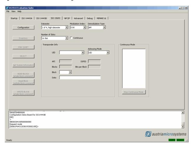
Once the board is configured to operate in the ISO15693 mode, the number of slots is set and *Inventory* button has to be clicked. The result of Inventory command is shown in the picture below (UID is presented).
