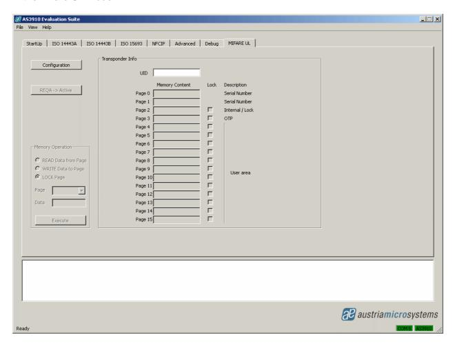
After clicking the button *Configuration*, a Mifare UL tag can be placed close to the demo board antenna. The button *WUPA->Active* starts the activation procedure and the UID number of the founded tag is displayed. In case more than one tag is detected during the *REQA->Active* command, the message "More then ONE transponder" is presented
