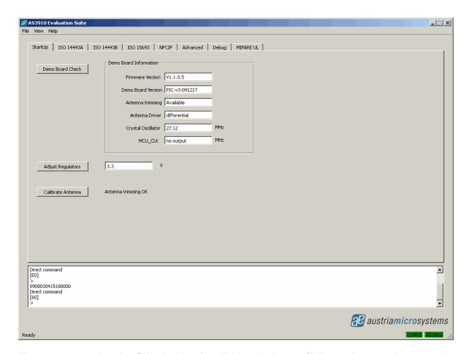
Figure above depicts the GUI window after clicking the button *Calibrate Antenna. Antenna trim-ming OK* is displayed next to the button.
