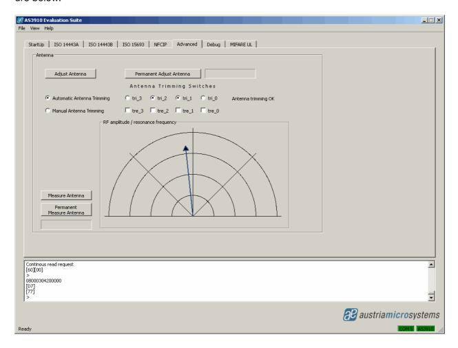
Measurement of resonance frequency can be done by the button *Measure Antenna*. Figure below depicts measurement result after placing some metal close to the antenna. In this case the antenna is not in resonance anymore (due to change of its inductance).
