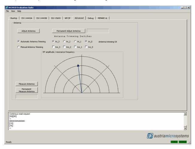
It is possible to define the position of trim switches and observe the effect on the resonance frequency. This is done by selecting *Manual Antenna Trimming* and defining the value of tre\_3 to tre\_0 before clicking button *Adjust Antenna* (check box marked indicates that switch is turned on).
