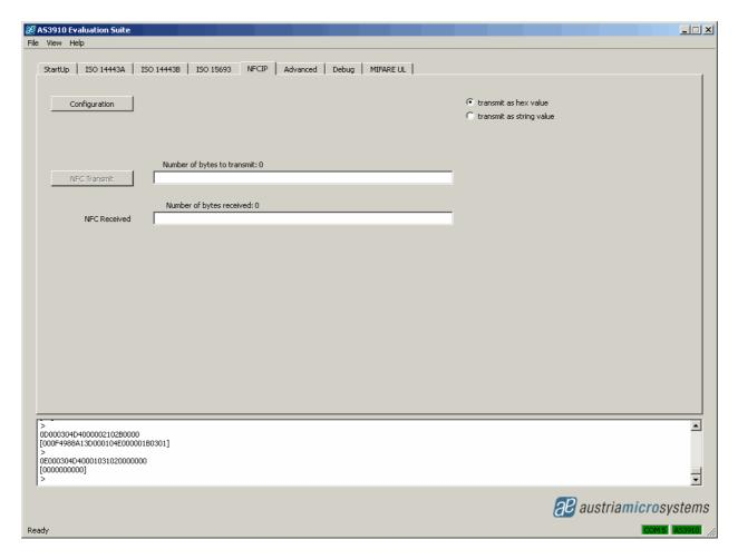
After entering *NFCIP* tab, the button *Configuration* has to be clicked. This configures the AS3910 in the NFCIP mode.
