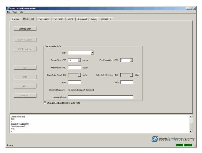
After clicking the button *Configuration*, an ISO14443A tag can be placed close to Demo board antenna. The button *REQA->Active* starts the anticollision procedure and the UID number of the founded tags is displayed.
