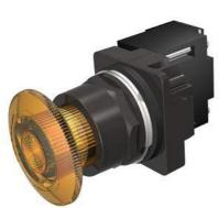
30mm BlackMax, Epoxy Coated Corrosion Resistant Metal Operator, Round Illuminated Twist-to-Release Transformer type, 480V AC LED Lamp Mushroom Head Cap Small 1.79" (45 mm) Plastic Cap, Amber 2 Position Maintained, Twistto-Release UL Listed, CSA Certified NEMA 1,3,3R,4,4X,12,13 & Automotive Standards
