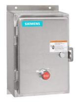
Non-reversing motor starter Size 1 Three phase full voltage Solid-state overload relay OLRelay amp range 0.25-1A 550/575-600 50/60HZ coil Combination type Water/dust tight non-corrosive
