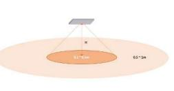
SEK-BLE-AOA can deliver both Azimuth and Elevation Angle estimates. That means one board can provide 2D X and Y coordinates. The actual positioning accuracy depends on the veritcal and horizontal distance between the board and BLE devices. The closer a BLE device is to the board, the higher positioning accuarcy it can achieve. For example, if the height difference between the board and a BLE device is H\*, then the coverage area and accuary will be like this:
