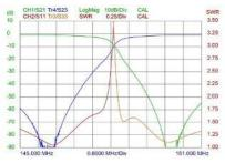
TYPICAL RESPONSE CURVES @ 8 MHZ DUPLEX SPACING
