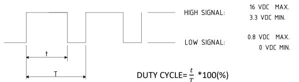
\*THE PREFERRED OPERATING POINT FOR THE FAN IS 25.0K HZ. \*AT 100% DUTY CYCLE, THE ROTOR WILL SPIN AT MAXIMUM SPEED. \*AT 0% DUTY CYCLE, THE ROTOR WILL SPIN AT MINIMUM SPEED. \*WITH CONTROL SIGNAL LEAD DISCONNECTED, THE FAN WILL SPIN AT MAXIMUM SPEED.
