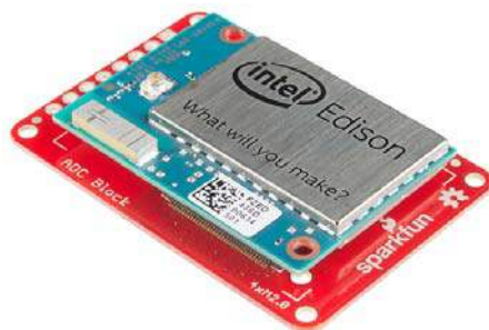
ADC Block Installed
