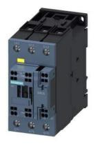
power contactor, AC-3e/AC-3, 65 A, 30 kW / 400 V, 3-pole, 21-33 V AC/DC, 50/60 Hz, with integrated varistor, auxiliary contacts: 1 NC, main circuit: screw terminal, control and auxiliary circuit: spring-loaded terminal, size: S2, F-PLC-IN
