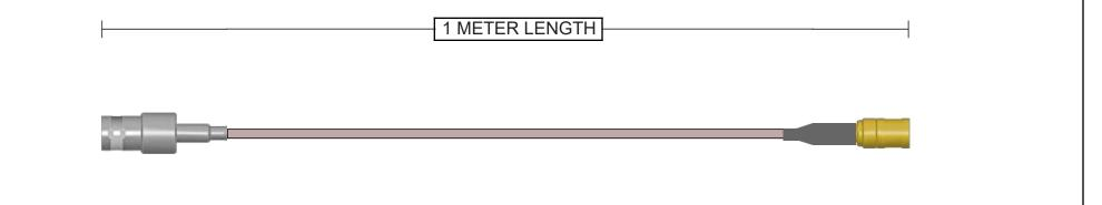
Connector A 112160 BNC Jack Straight Brass Nickel 50 Ohm RG-316 Continuity/Hi-Pot Connector B 142186 SMB Plug Straight Brass Gold + Heatshrink
