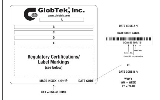
A=ICT/ITE Power Supply B=P/N: (料号) WR9MA1000USB1-F(R6B) C=Model (型号) GT-83083-0505-USB-W2E D=Input (输入)100-240V-, 50/60Hz, 0.2A E=Output (输出)5.0 V == 1.0 A, 5.00W
