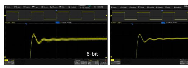
10-bit mode combined with Zoom shows you more details and less noise on the waveform.
