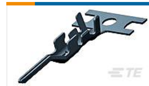
TE Part #2238007-1 TERMINAL, PIN, LANCELESS, 22-26 AWG, EP2
