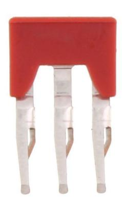
Insulated cross-connector, No. of poles: 3, Mounting type: Plug in, Width: 14.2 mm, Rated cross-section: 2.5 mm², Colour: Red
