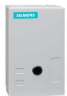
Non-reversing contactor, Size 1P, Single phase full voltage, Contactor amp rating 35A, 3 wire (NO aux included), 208VAC 60Hz coil, Non-combination type, Enclosure NEMA type 1, Indoor general purpose use, Standard width enclosure
