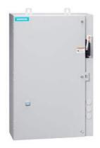
Non-reversing motor starter, Size 3, Three phase full voltage, Solid-state overload relay, OLR amp range 25-100A, 240V 50Hz / 277V 60Hz coil, Combination type, 200A fusible disconnect, 200A/250V fuse clip, Enclosure NEMA type 4/12, Water/dust tight for outdoors, Extra-wide enclosure
