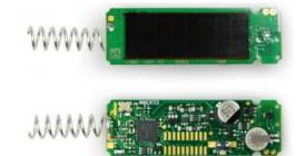
Power is provided to STM 350 by means of a small pre-installed solar cell which works in conjunction with an integrated energy storage element in order to ensure operation in periods without ambient light.
