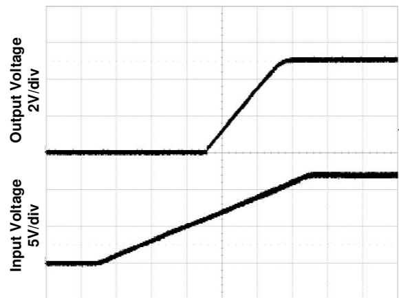
Figure 5. Start-Up from Enable Vin = 12V, Vo = 5V, Io = 0A Control
