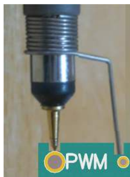
Figure 4. Recommended Use for Ground Spring Clip Test Points
