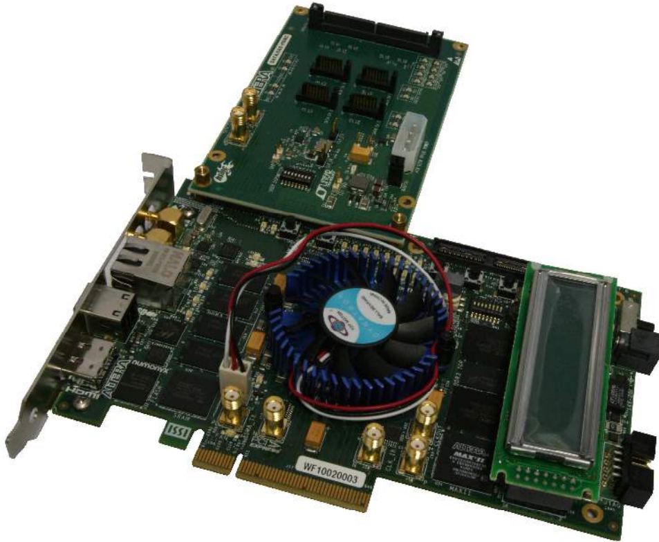
Figure 4.3 Connecting the SATA/SAS daughter card to the Stratix IV development board
