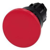
$\label{eq:mushcompushbutton, 22 mm, round, plastic, red, 40mm, momentary contact type, with laser labeling, lower case$
