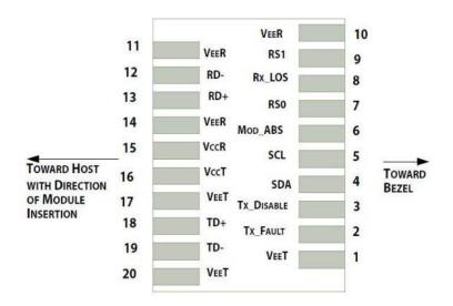
Pin-out of connector Block on Host board
