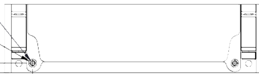
RECOMMENDED HOLE LOCATIONS FROM PCB EDGE SCALE 1 : 1
