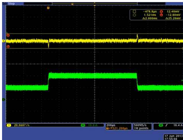
FIGURE 13. STEP RESPONSE, 10A TO 20A AT 5A/µs, ASCR = 1000 TOTAL DEVIATION WINDOW 25mV = 2.5%
