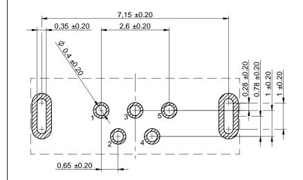
CHECKED REVISION DATE (YYYY-MM-DD) GENERAL TOLERANCE PROJECTION METHOD Đ G BaBo 001.001 2022-04-05 DIN ISO 2768-1m 0 ΡĽ DESCRIPTION RoHS COMPLIANT REACH HALOGEN Micro USB 2.0 Type AB Vertical 5 Würth Elektronik eiSos GmbH & Co. KG **Contacts** ORDER CODE EMC & Inductive Solutions WURTH ELEKTRONIK Max-Eyth-Str. 1 614105150621 74638 Waldenburg Germany MORE THAN YOU EXPECT Tel. +49 (0) 79 42 945 - 0 www.we-online.com STATUS BUSINESS UNIT PAGE 1/6 eiCan Valid eiSos@we-online.com
