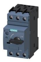
Circuit breaker size S0 For system protection Without phase failure protection Arelease 18...25 A Short-circuit release 325 A Screw terminal Standard switching capacity
