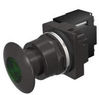
30mm BlackMax, Epoxy Coated Corrosion Resistant Complete Metal Unit Illuminated Push-Pull Operator Transformer type, 120V AC LED Lamp Mushroom Head Cap Small 1 3/4" (44.5 mm) Metal, Black with Green Lens 3 Position Pull-Momentary/Push-Maintained UL Listed, CSA Certified NEMA 1,3,3R,4,4X,12,13 & Automotive Standards
