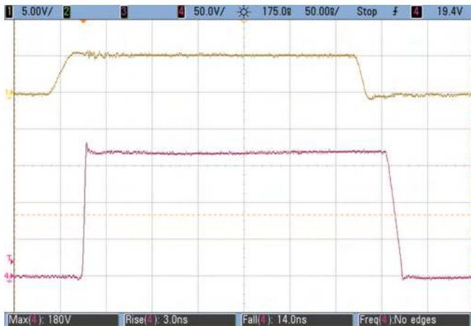
Figure 4: Waveforms for V_{IN} = 170V to 5V/5A (100kHz) Buck converter CH1: V_{PWM} Input voltage – CH4: ( V_{OUT} ) Switch node voltage
