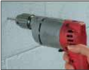
1. Drill hole using correct size bit.
