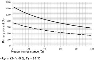
$U_C = \pm 24 V - 5 \%$ ,  $I_A = 85 °C$ ---  $U_C = \pm 15 V - 5 \%$ ,  $T_A = 85 °C$ Primary currents higher than  $I_{PM}$  only for peak!
