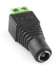
**Description:** This adapter allows you to connect a barrel jack connector to bare wires. One end has screw terminals and the other has a 5.5x2.1mm, center-positive female barrel jack. If you have a power supply with a barrel jack and want to plug it into a breadboard, this might be the simple solution.
